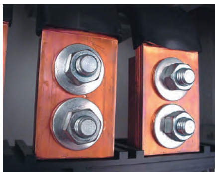
Connection of a 50 x 10 bar using two M12 screws Cat.No 0 374 65 with integrated wide washers
