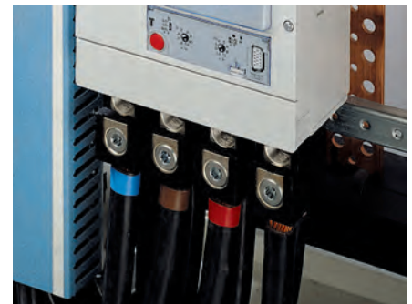
Connection of two aluminium conductors (185 mm 2 per pole) to a DPX 3 630 with terminals Cat.No 0 261 51
