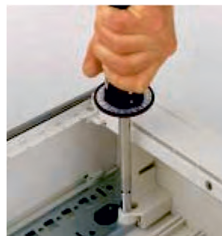
Example: checking the tightening torque.
