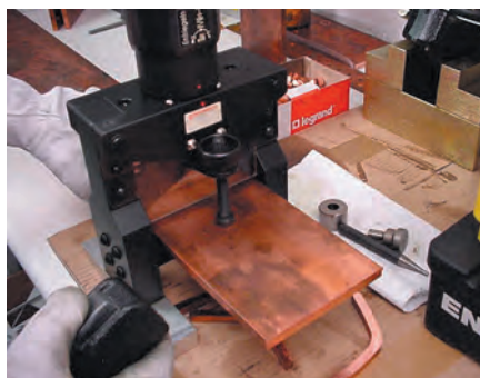
Bending a 10 mm thick copper bar on a portable hydraulic tool
